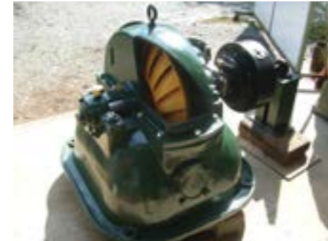
Above: 53.7kW Turgo installed 1920 at Rydal Hall Ambleside
