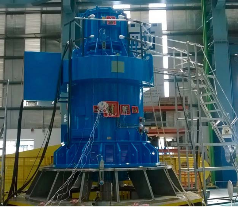
Generator during factory testing
