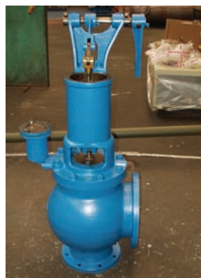
Refurbished dashpot relief valve in Gilkes factory
