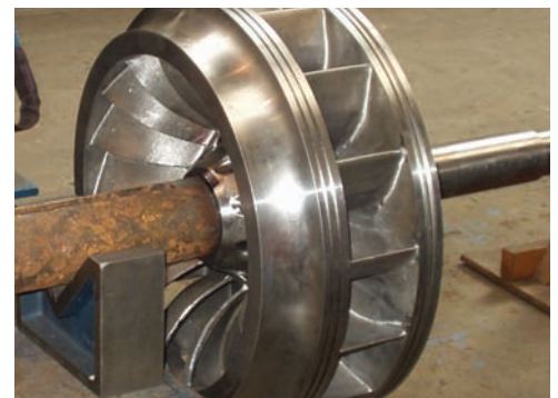
Replacement Stainless Steel runner on original/modified turbine shaft.
