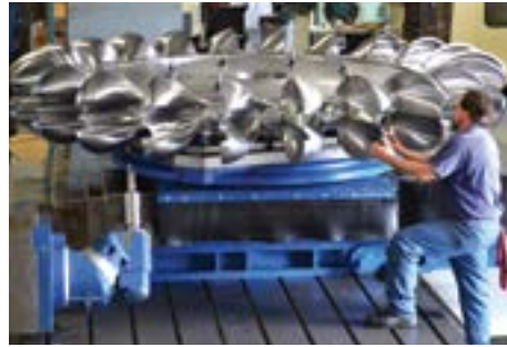
Above: Inspecting a one-piece, 7 MW Pelton runner on Canyon's 7-axis CNC mill. The runner has a diameter of 3.4m (11.25ft) and weighs 21,000 pounds. The computerized milling process creates an exact match of the digital 3D model created during design.
