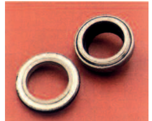
Mechanical Seal: Carbide or graphite/ceramic with automatic lubrication. Can run dry and operate on high vacuum even with abrasive liquids
