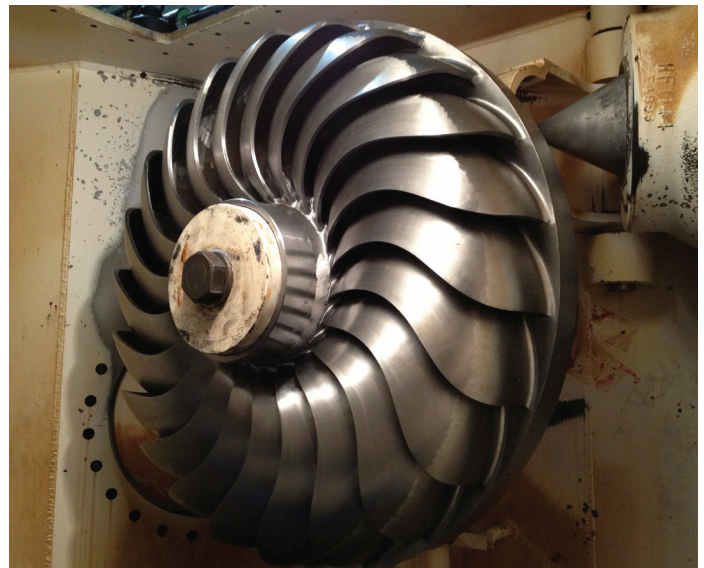
New CNC machined runner installed
