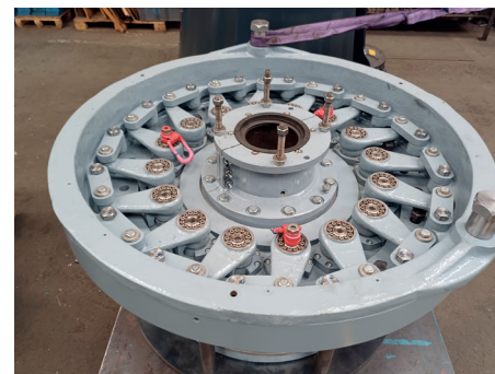
Below: Redesigned guide vane mechanisms for Glen Finglas refurbishment
