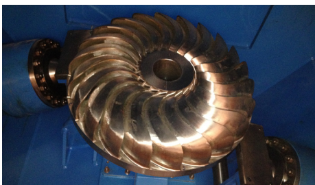
Runner & Spear Valves inside case
