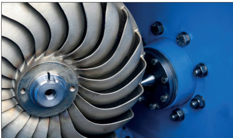
(a) A 10.5 in (27 cm) Turgo runner with spear and nozzle design in the background.
