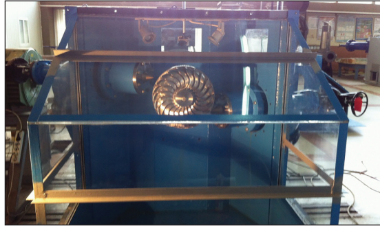
(c) Gilkes Turgo test rig at NTUA, Athens.
