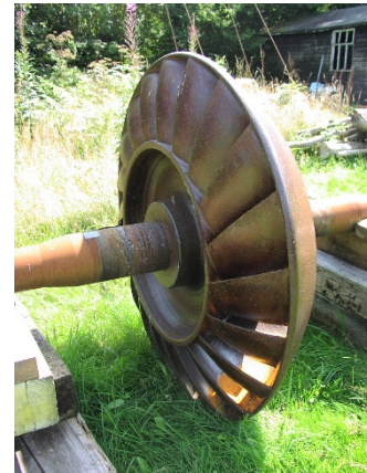
A Turgo runner to the 1919 design taken out of service after 70 yrs. There was very little wear!
